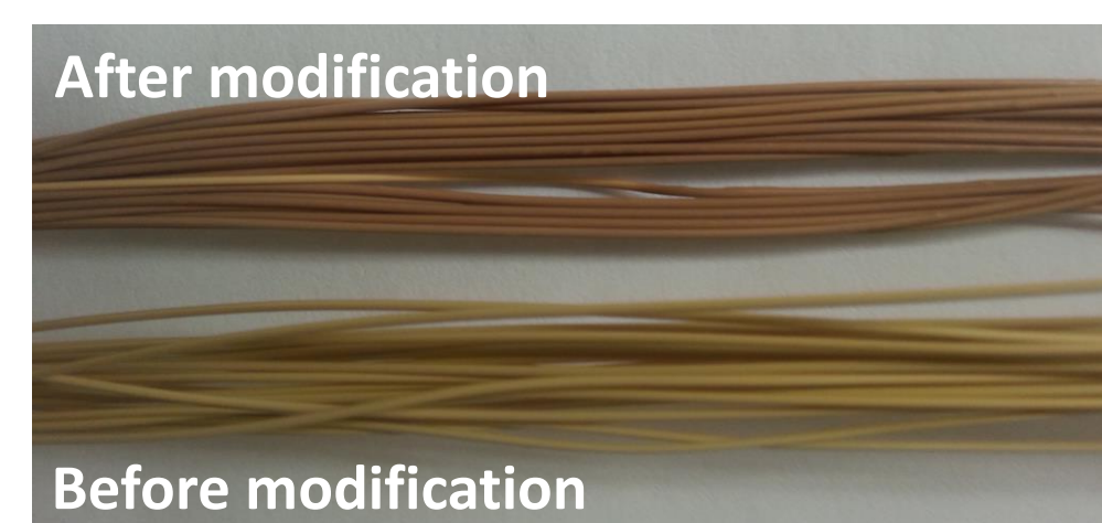
Figure 4. Color change of PBI fibers after modification to lower pKa.
